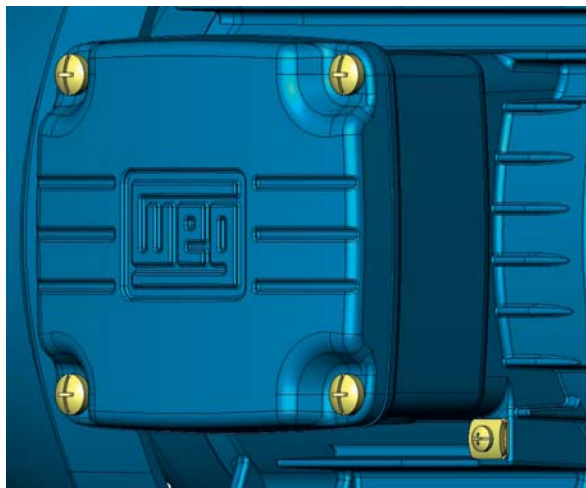
Figure 2 - Detail of the grounding lugs on the frame
